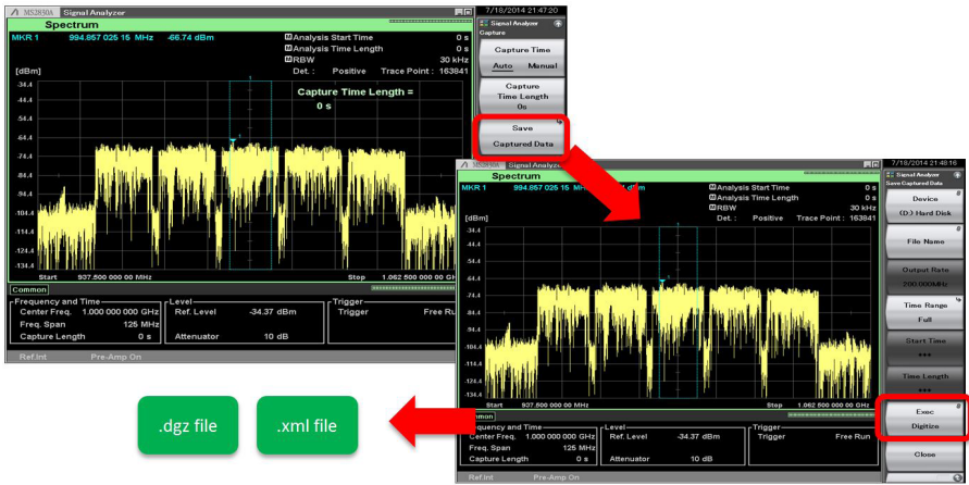
Fig 55 - Capturing real 5G waveforms with MS2830A
