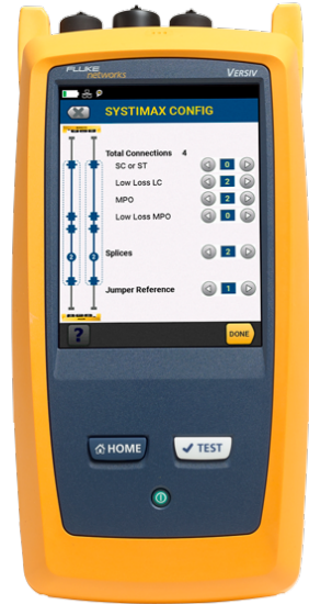
Figure 3. The CommScope SYSTIMAX Link Loss Calculator is built-in to the latest version of Fluke Networks CertiFiber Pro Optical Loss Test Set. CertiFiber Pros owners can add the calculator to their testers with a free download from the Fluke Networks website.
