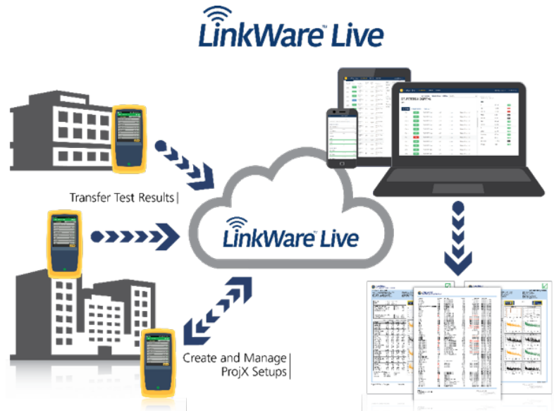
Figura 4. With LinkWare Live, Project Managers can create and manage test settings and transfer them to testers. Techs can upload test results, allowing the Project Managers to track job progress.
