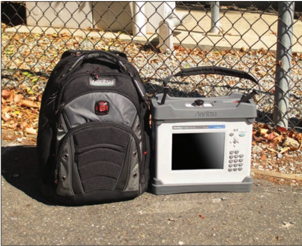
PIM Master MW82119A 40 Watts, Battery-operated
