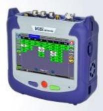
The MTX150 is a fully-integrated and self-contained multi-service test solution for OTN, SDH, SONET, PDH, DSn, Ethernet, SyncE, Mobile Backhaul, and Fibre Channel (SAN). This all-in-one, rugged and ultra-portable field hand-held test set can be configured with interfaces and technologies required by field technicians to install, verify, maintain and troubleshoot Transport, Metro, Access communication links and services, including legacy applications.
