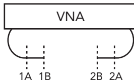
Figure 52. According to the reference plane concept, if adapters, fixtures and cables are added/changed after a calibration, distortions can result.
